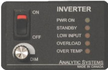
A remote control panel may be connected to the inverter using a 9-pin D connector, which attaches to the front panel of the inverter. The remote control panel and D connector are part of the remote control option. The remote control panel allows the unit to be operated remotely as well as duplicating all the diagnostic indicators and audible alarm.
